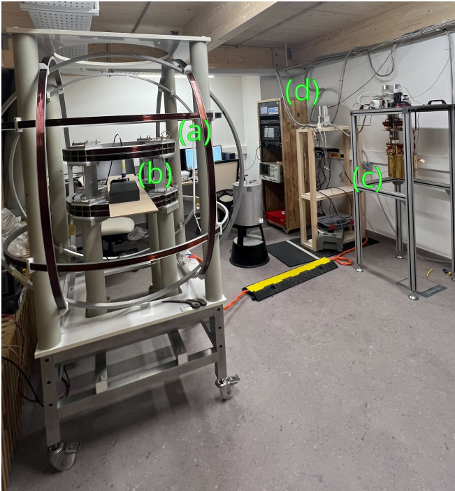
FIG. 3. The Atlantic 10 mT prototype. Like Pacific, the B_0 field is generated by a 40 A current, here through a smaller copper solenoid (a). The sample is placed between the gradient plates and main coil (b). The MRI signal is picked up by a room-temperature copper coil around the sample and sent inside the cryostat (c) where it is amplified by a low- T_c SQUID (SQ2600, STAR Cryoelectronics). In this case, the cryostat is open, revealing the gold-plated structure that cools the SQUID. In later iterations, this room-temperature pickup coil will be cooled with the custom cryostat described in Fig. . The signal is then read out by room-temperature electronics in the rack (d).
