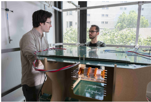
FIG. 27. Discussions inside the B0 coil, the big PCBs serve as gradient plates. The RF transmit coil and pickup coils can be seen between the PCBs.
