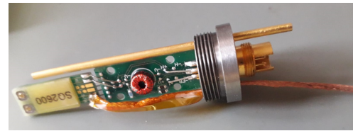
FIG. 17. A SQUID magnetometer, model SQ2600 of STAR Cryoelectronics mounted with readout electronics and a Niobium shield assembly (shield open on the picture). The SQUID chip is protected under the resin layer on the left side of the picture. The input coil can be accessed through the two Niobium pads, leads are introduced in the shield through the thin metallic tube on the top. We use a copper thread as a heat sink to properly thermalize the chip, by connecting it to the cold plate of the cryostat.
